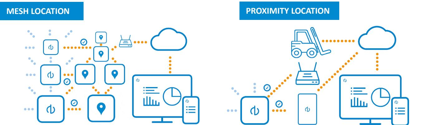
A system consists of a mesh gateway and a number of tags - either configured as anchors or asset tags. Anchors are attached to walls and automatically forms an industrial mesh network. Asset tags regularly use the mesh network to automatically provide its location.
