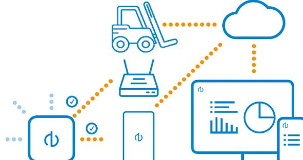
The tag is configured to also advertise its presence using BLE-beaconing. This makes the tag readable also for stationary gateways, mobile gateways and smartphone apps.
