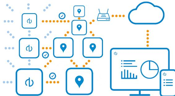
A system consists of a mesh gateway and a number of tags - either configured as anchors or asset tags. Anchors are attached to walls and automatically forms an industrial mesh network. Asset tags regularly use the mesh network to automatically provide its location.
