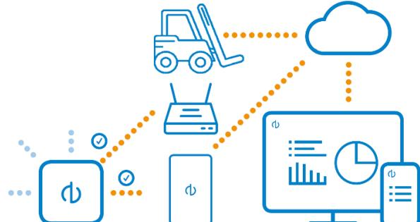
A system consists of a mesh gateway and a number of tags - either configured as anchors or asset tags. Anchors are attached to walls and automatically forms an industrial mesh network. Asset tags regularly use the mesh network to automatically provide its location.
